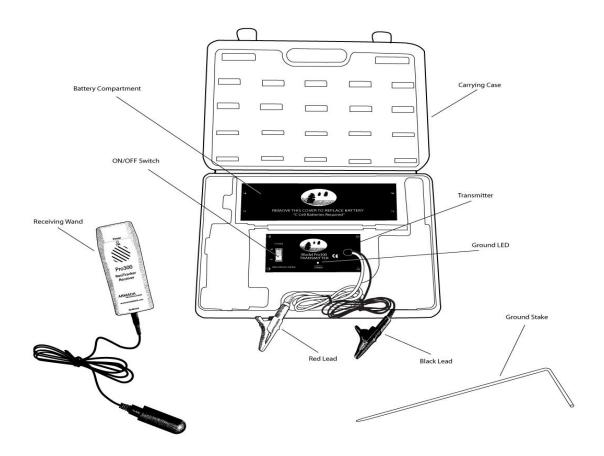
The Armada Technologies Pro290 wire and cable locator is designed to find lost or broken wires, and trace their paths. The complete Pro290 kit consists of;
