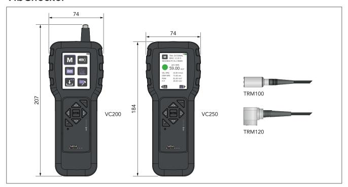
VibChecker is an instrument for fast and easy measurement of machine condition in preventive maintenance. It is based on the recommendations of ISO 2372 and ISO 10816 standards for broad band measurements of vibration. These standards make the assumption that limited information, obtained easily and at a low cost, is often as useful as a detailed analysis using expensive equipment and elaborate techniques.
