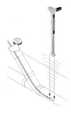
that it produces a "null" (signal strength very close to zero), and then counter-rotate 90 degrees to go back to the original position.
