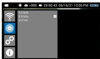
Fig. 29: Locator detection with 8.9 kHz transmission frequency selected
