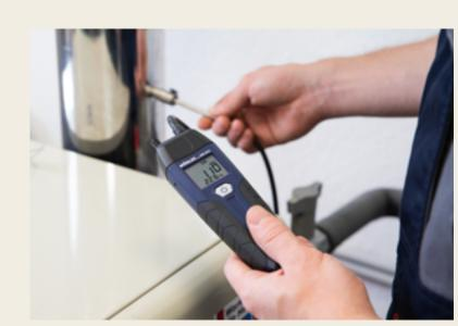
With the Wöhler DM 602, you can work both quickly and precisely when taking settings from the burner and when measuring the draught in the flue gas pipe.
